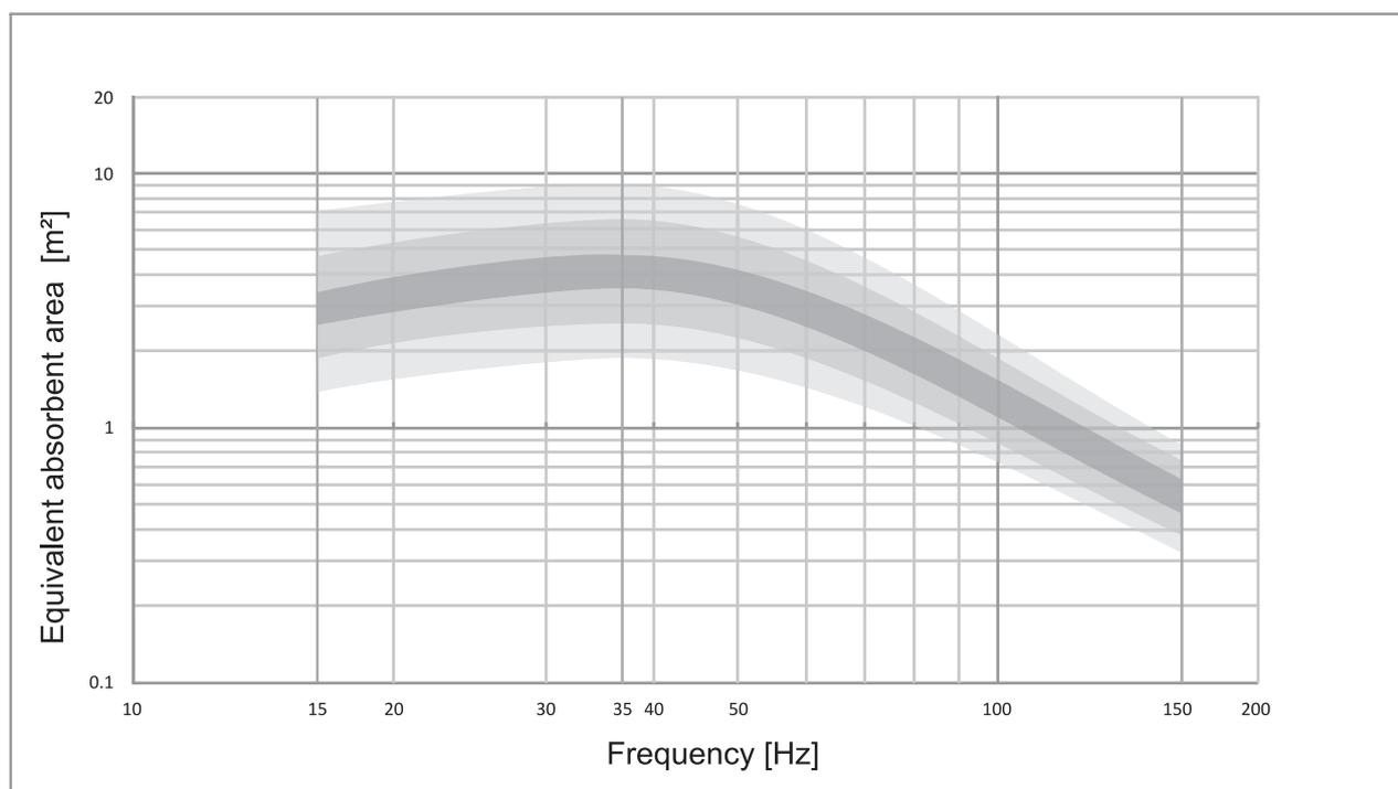
Note that in normal operating conditions the AVAA does not emit any audible sound or anti-noise but only absorbs low frequencies in an very effective way considering its size. Furthermore, it has no impact on the direct sound from your speakers or other source.
