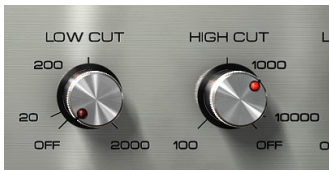
Figure 11: The Low and High Cut knobs.
